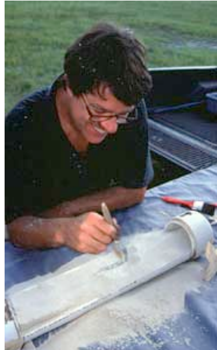
McCollum excavates his fulgurite from the PVC pipe “Pod” used as a receptacle for receiving the lightning strike at Camp Blanding.
