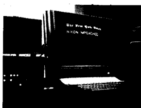
Responding computer displays come in all sizes and prices. This little setup (in the under-$10,000 class) is a PDP-8 minicomputer with home-built display circuitry. Gothic lettering data structure available from somebody in the military; message courtesy of R.E.S.I.S.T.O.R.S. The big display is an IBM 2250 (over $100,000, including minicomputer).
